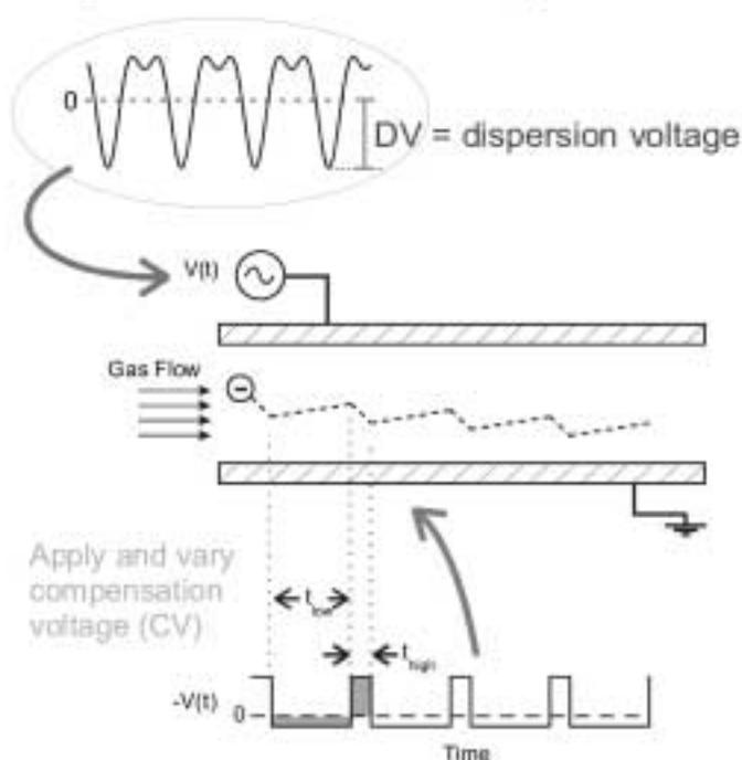
Figure 3 Schematic of FAIMS operation
