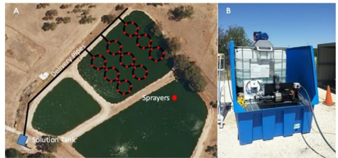
Figure 1: Wastewater lagoon hydrogen peroxide delivery system (A) with mixing tank and pump (B).
