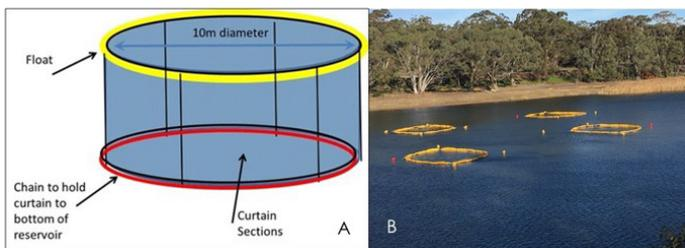
Figure 4: Mesocosm design (A) and reservoir installation (B).
